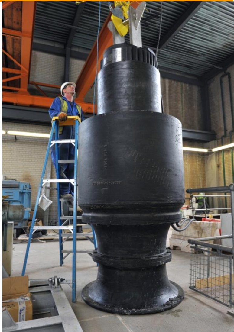
Bedford Pumps' Storm Pump for Ashton Avenue
