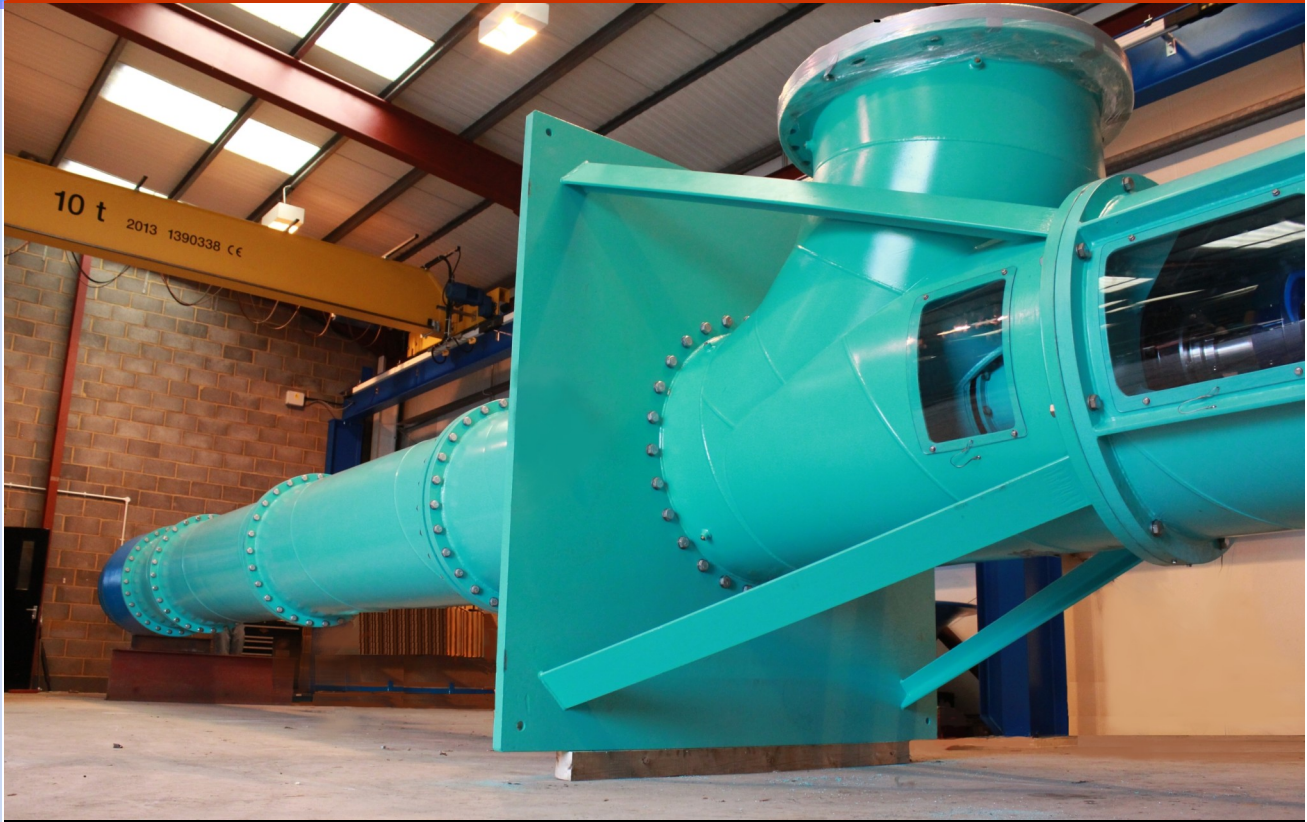
Suspended bowl pump for Toll House SPS at Bedford Pumps' works
